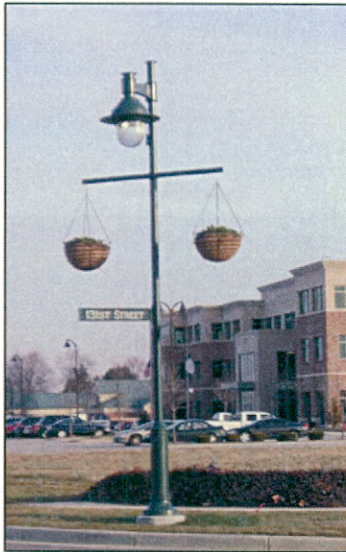
Multi-functional streetlight incorporating street signs and hanging baskets.
