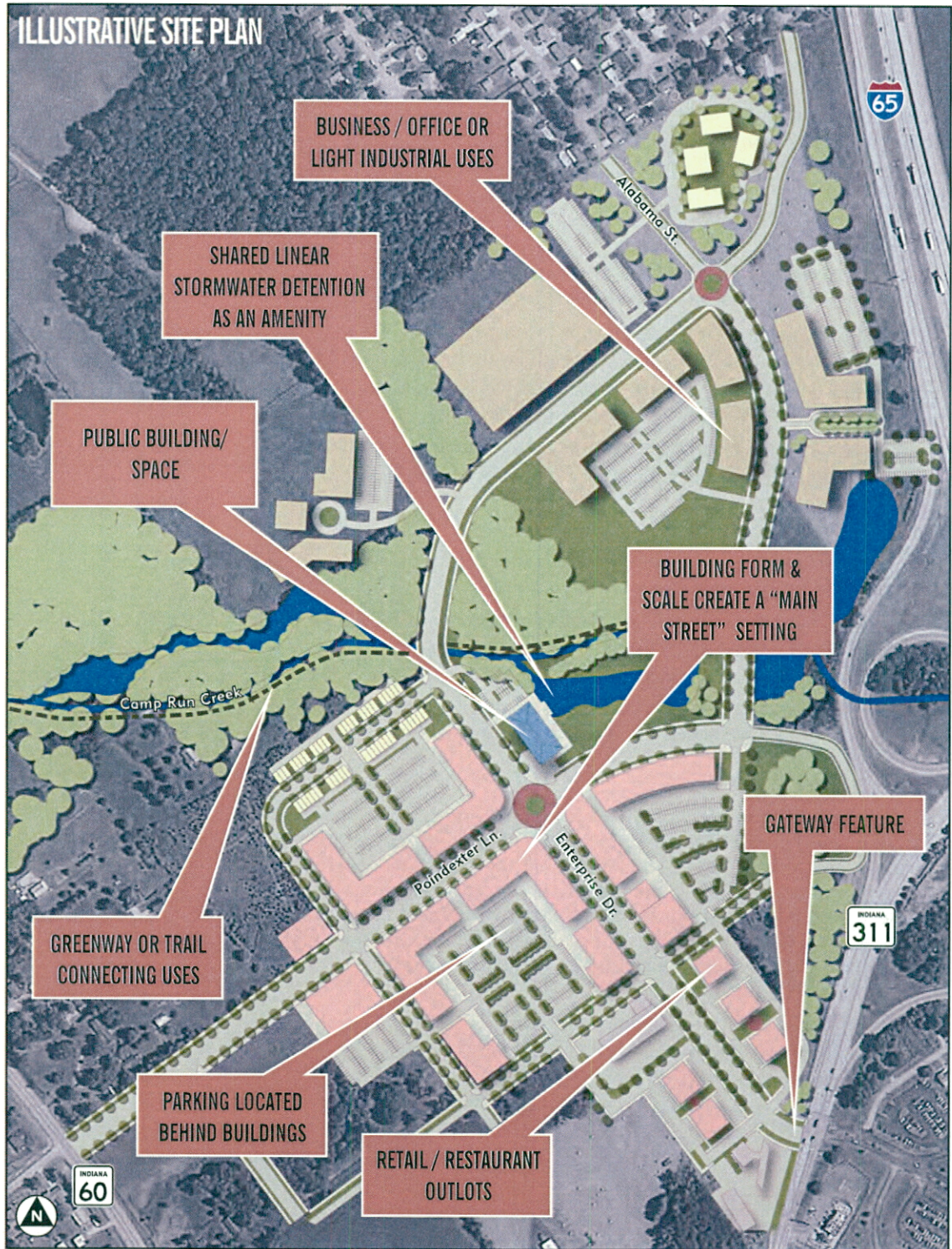
Illustrative Site Plan of one potential concept focused on core and interstate areas
